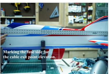
Start by temporarily installing the rudder with the control horn installed. Install the rudder servo with it control arm. Now you can mark a line on the outside of the fuse at the height of the servo arm (see photo 1). Just visually sight it and make the mark.
