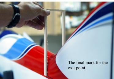
with 2" for the holes. the inside dimension of the tool is 2". Using that tool, slide it over the rear fuse and mark where it
