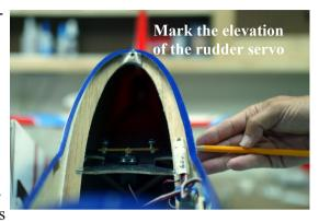
outside holes 2 inches apart so the holes on the control horn on the rudder need to be 2 inches from hole to hole if you use that servo arm.
